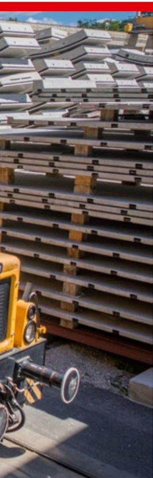
An essential criterion here is the precision of the end product, the segment ring. Because of accuracies of  $\pm 0.3$  mm, production facilities, manual skills and engineering services in planning and execution are required at the highest level on a daily basis.
