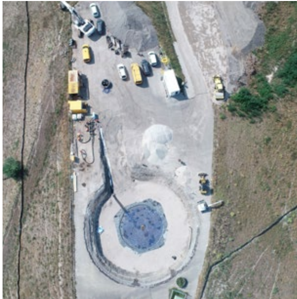
Ground freezing for stabilizing a foundation on a landfill
