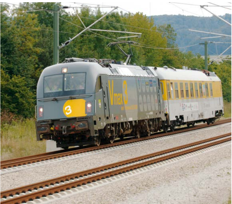
World record on FF Bögl between Nuremberg and Ingolstadt: In a speed of 357 km/h, the "Taurus III" locomotive set a new speed record for electric locomotives on a non-prepared track.
